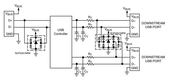
Figure 10. ESD Protection for USB Port
