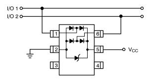
For this configuration, connect pin 5 directly to the positive supply rail ( $V_{\rm CC}$ ), the data lines are referenced to the supply voltage. The internal surge protection diode prevents overvoltage on the supply rail. Biasing of the steering diodes reduces their capacitance.
