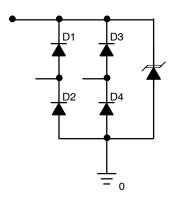
Figure 9. NUP2201MR6 Equivalent Circuit
