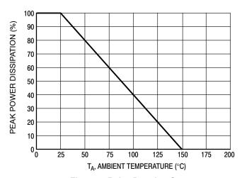
Figure 6. Pulse Derating Curve
