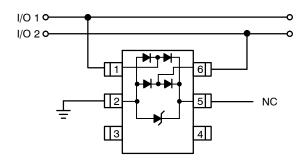
In applications lacking a positive supply reference or those cases in which a fully isolated power supply is required, the internal surge protection can be used as the reference. For these applications, pin 5 is not connected. In this configuration, the steering diodes will conduct whenever the voltage on the protected line exceeds the working voltage of the surge protection plus one diode drop  $(Vc = Vf + V_{RWM})$ .
