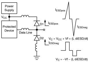
An approximation of the clamping voltage for these fast transients would be:
