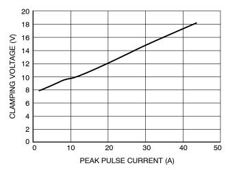
Figure 8. Clamping Voltage vs. Peak Pulse Current (8 x 20 µs Waveform)
