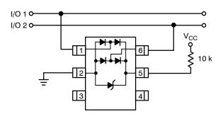
The NUP2201MR6 can be isolated from the power supply by connecting a series resistor between pin 5 and  $V_{CC}.\ A$  10  $k\Omega$  resistor is recommended for this application. This will maintain bias on the internal surge protection and steering diodes, reducing their capacitance.
