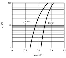
Source-Drain Diode Forward Voltage
