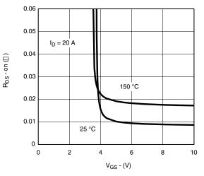
On-Resistance vs. Gate-to-Source Voltage
