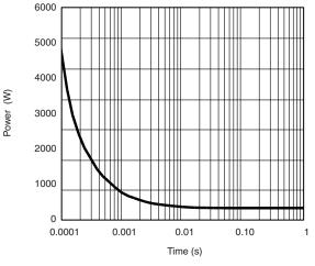
Single Pulse Power, Junction-to-Case (T<sub>C</sub> = 25 °C)
