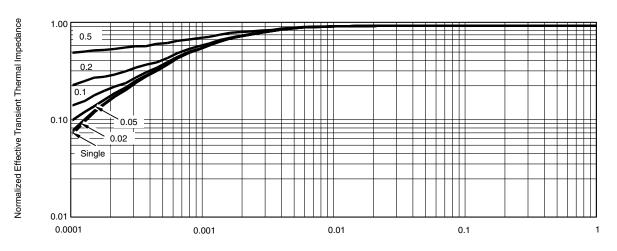
Normalized Thermal Transient Impedance, Junction-to-Case
