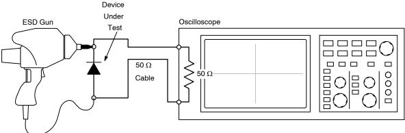
Figure 4. Diagram of ESD Test Setup
